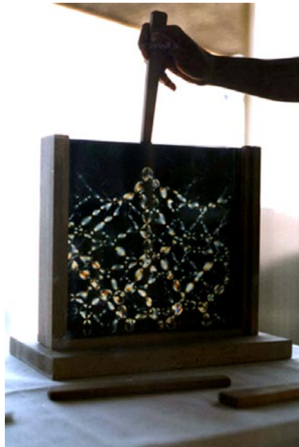
Figure 1. Force chains through a disordered granular packing made by a mixture of photoelastic discs with two different sizes. The luminosity is proportional to the amount of stress carried (see footnote 3 below).
